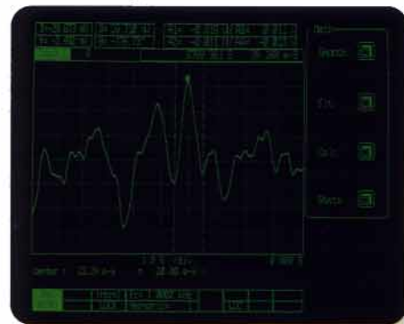
Figure 3 - Chart display allows on-screen data recording (64k points).
