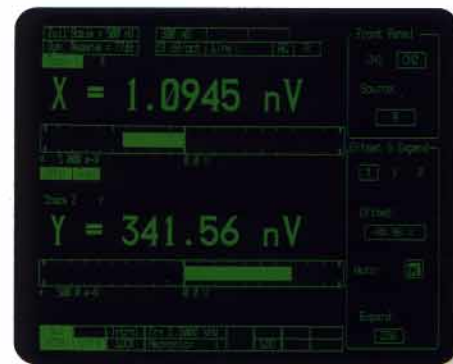
Figure 1 - Bar graph and numerical read-out resembles a conventional lock-in display.
